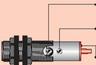
► **TRIMMER FOR THE SENSING RANGE ADJUSTMENT:** The photocell is supplied with max. sensing range with the trimmer totally rotated in the clockwise direction. The sensitivity reduces by rotating the trimmer in the anti-clockwise direction.
